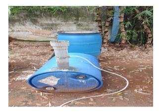
GASTODAY equipment produces cooking gas from leftover domestic or home based food/vegetable/organic waste through the process of anaerobic bacterial digestion in simple terms, the organic waste is degraded biologically, and biogas which is produced as output, is used for cooking.
